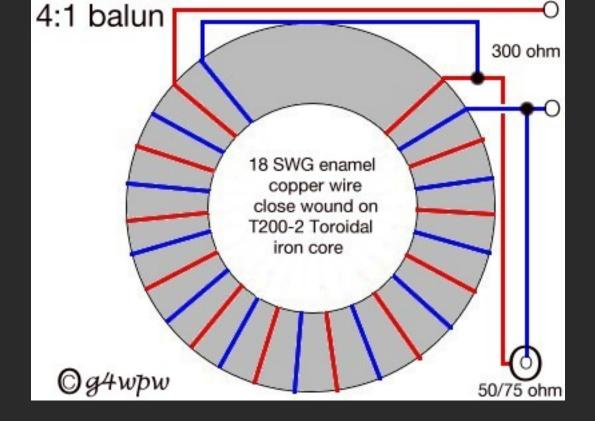
a small gap must be left between the start and finish of the windings
