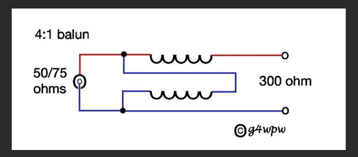
The construction for this balun uses the same principles as the previous one use a 300 ohm carbon resistor to check the swr,this should again be 1:5 - 1 or less.
