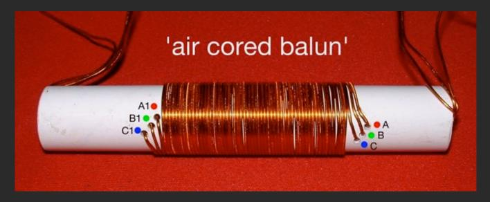
The finished balun's should be encased or insulated from the elements.
